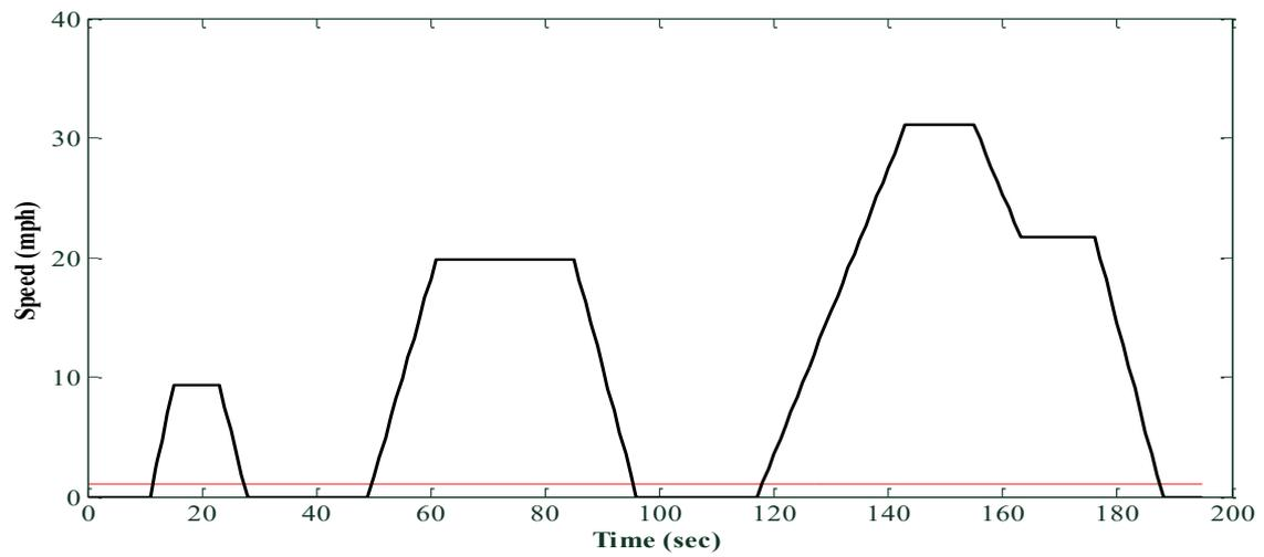
**Figure 3: FTP Drive Cycle**
