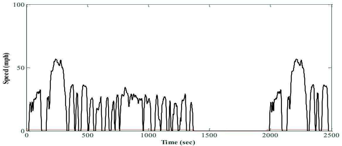
**Figure 4: HWFET Drive Cycle**
