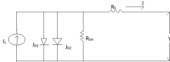
$$I_{sh} = \frac{V}{R_{sh}} \cdot \frac{N_p}{N_s} + \frac{I}{R_{sh}} \cdot R_s \quad (1)$$
