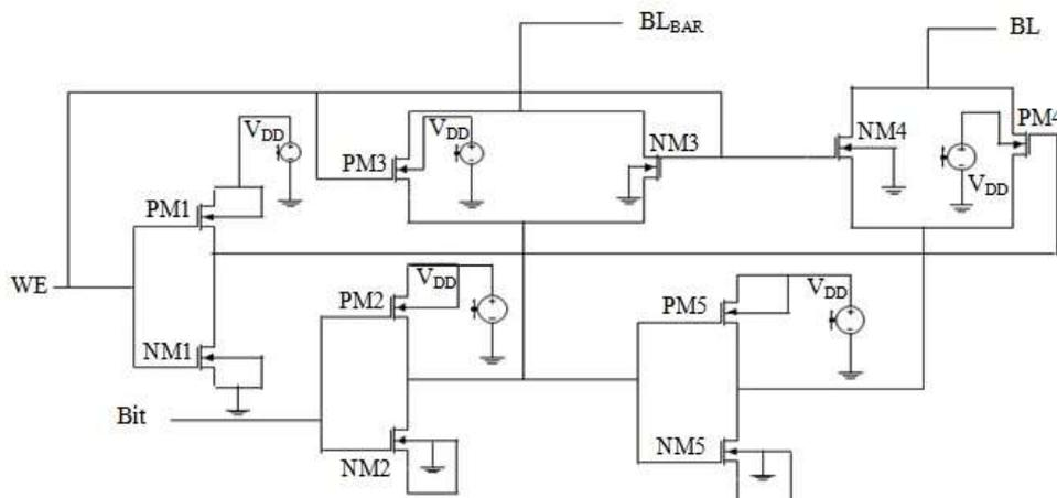
Figure 2 depicts the NM3 and NM4 driving transistors for a STSRAM cell. One of the transistors in this circuit is the driving transistor. These bit lines widen the noise margin. Researchers can calculate how much voltage can fluctuate by using a differential circuit. As long as the present
