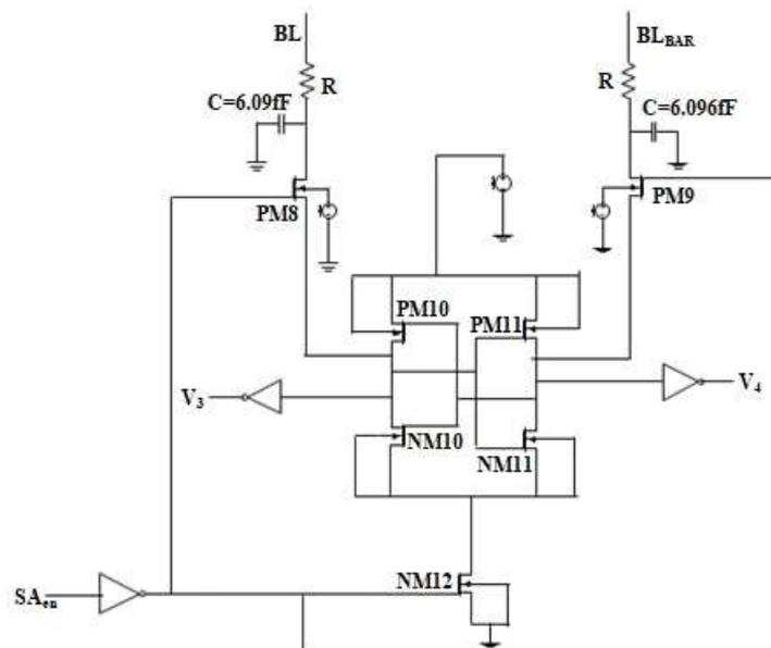
The circuit's building blocks, the nodes, manage the input bit lines. When the word line is lifted, the amplifier sensor fires, but PM8 and PM9 are not engaged. The voltage differential impacts the random bit voltage in the internal nodes of the LSA between the bit lines. When the LSA SAEN signal is claimed, the greater voltage difference between inverters boosts maximum swing power [22–25].
