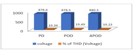
The graph on the right shows the total harmonic distortion (THD) as a percentage and the basic output voltage for each of the available methods. A variety of PWM approaches show how the fundamental voltage and the total harmonic distortion are affected by the different strategies. With all of the PWM approaches, harmonic distortion was fully eradicated.
