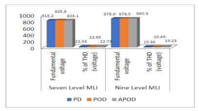
The results of a comparison between MLI levels seven and nine are shown in the graph included in this article. The graph shows that the fundamental output voltage increases as the overall harmonic distortion decreases for a total of nine level inverters. It's also clear from the graph that this is happening despite the fact that overall harmonic distortion has decreased.
