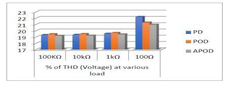
The load comparisons are shown in the graph above for your consideration. The THD count shows that when the load increases, the total harmonic distortion decreases as compared to its level when the load is modest. This is due to the fact that one of the several PWM algorithms is used to calculate the THD count.
