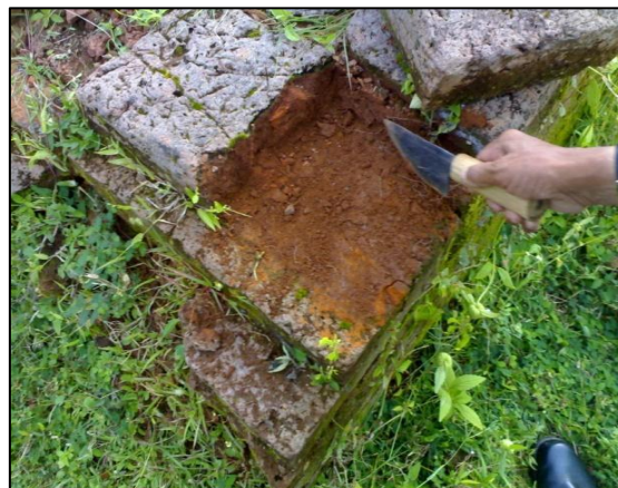
Fig 3: Collection of Mortar Sample
