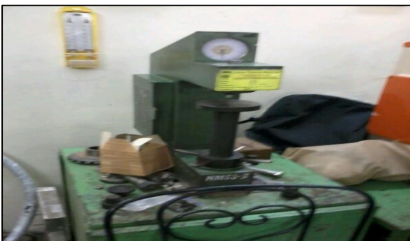
Fig 3: RESULT: the Rockwell Hardness Test Gave 25-26 HRC
