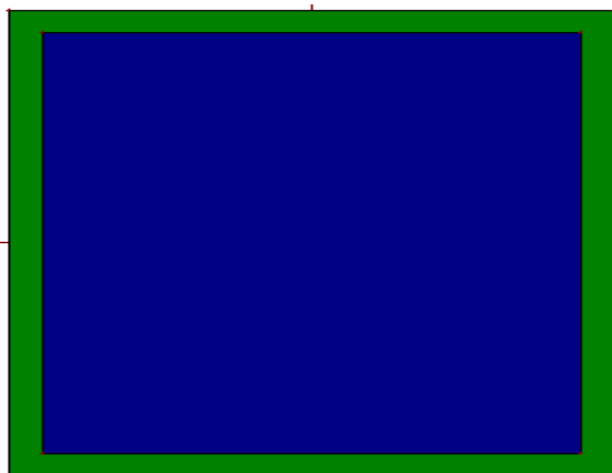
Fig: 1. Microstrip Rectangular Patch Antenna
