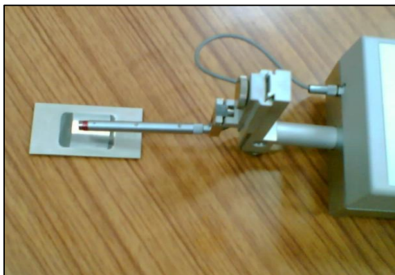
Fig 10: Calibrating view with Measuring Instrument (Surtronic 3+)
