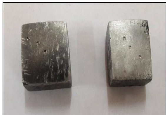
Fig 12 MMC Sample After Indentation on Hardness Testing Machine
