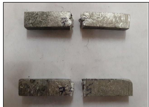
Fig10: MMC sample After Toughness Testing
