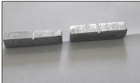
Fig 12: MMC sample prepared for microstructure
