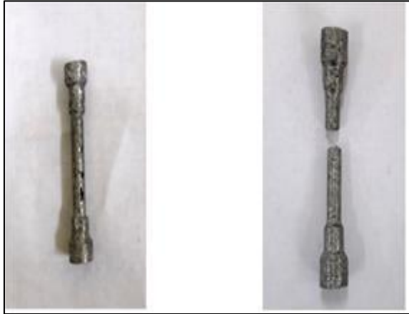
Fig 6: Tensile Test of 2.5% of Al 2 O 3 Mixed with Al
