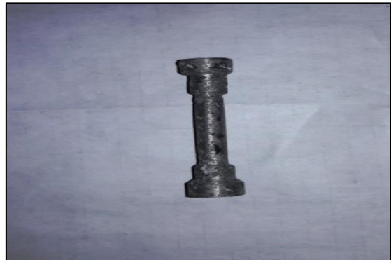
Fig 11: MMC Sample Prepared for Toughness Test
