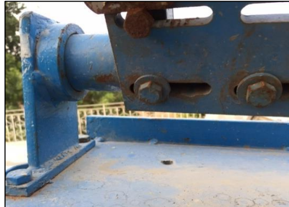
Fig 2: (b) – Mechanism to Slide Motor Plate to Vary Gap Between Wheels
