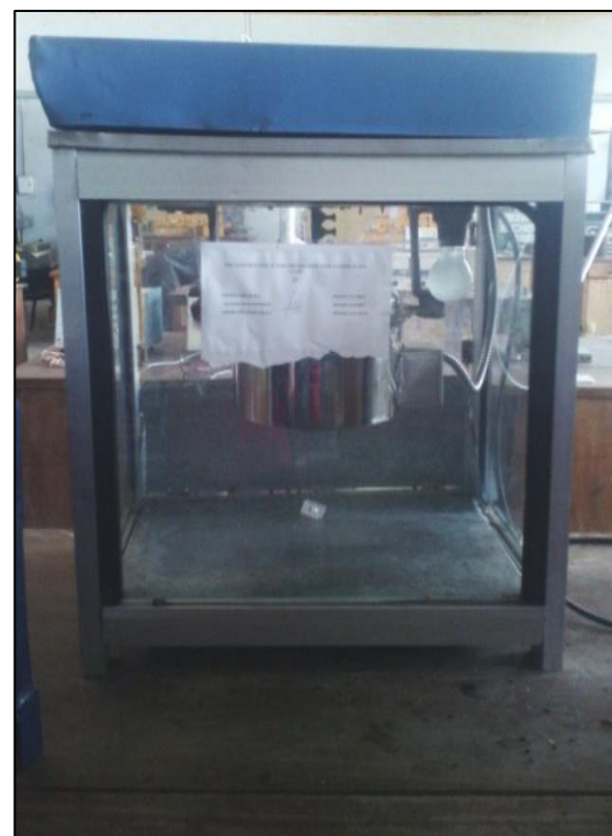
Fig 7 (a): Machine with Aluminium and Glass Compartment
