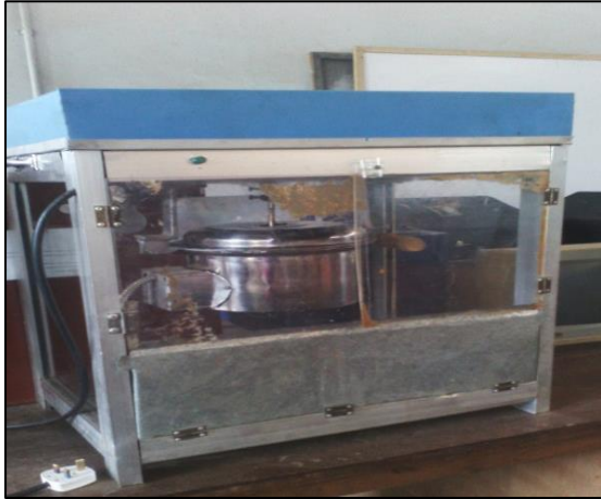
Fig 7 (b): Developed Pop- Corn Machine
