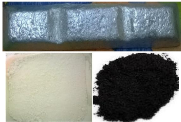
Fig 1: Aluminum 7075 Alloy ingot, TiO 2 Powder and Graphene Oxide Powder
