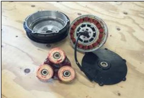
**Figure 2: Direct-Drive Motor**
