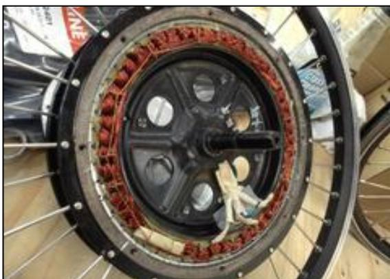
That normally means more weight, and the hills are very long. So, for twin bikes, cargo bikes, or riders that weigh more than 100kg, we have a direct drive engine. When you coast, there is a tiny bit of resistance generated by a direct drive engine. By operating the motor on a tiny trickle of power, this can be absolutely avoided.
