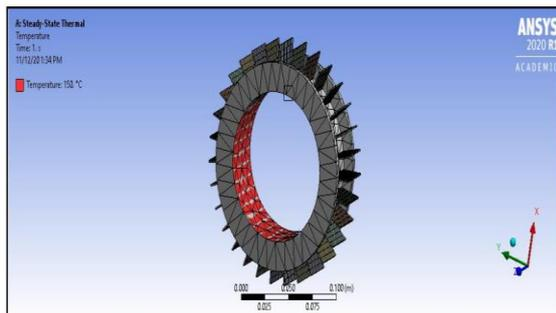
After the meshing the temperature boundary conditions were set to 150 °C on the inner part because the max heat which can be dissipated from the hub motor is 150 °C as per the operating condition of Motor operated Hub wheel
