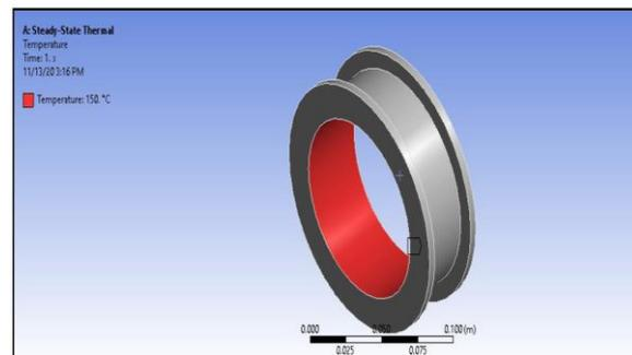
The temperature must be applied in the inner surface of the circular model by changing the magnitude temperature to 150 degrees. As the atmospheric temperature is applied in this case in order to kept this model based on convective heat transfer. And the film coefficient and Stagnant Air-Simplified Case has been considered for the final investigation based on heat transfer aspects.
