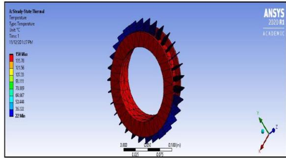
The red zone represents the heat dissipation and the blue represent the dissipation through fins and cooling the model.
