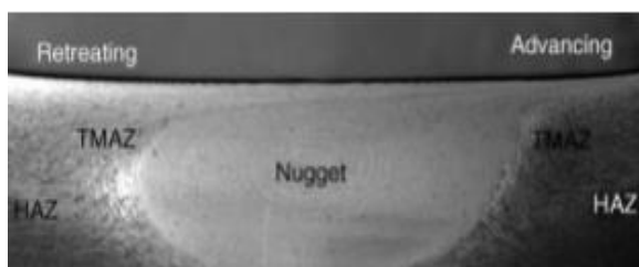
Fig 4: A Macrograph Showing Various Microstructural Zones in FSP 7075Al-T651 (Standard Threaded Pin, 400 rpm and 51 mm/min). [1]
