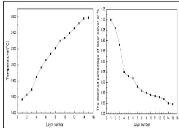
The model was used to simulate the entire 15-layer LDMD process. Temperature distributions with layer number were shown in Figure 16 (a) above under constant laser power condition.
