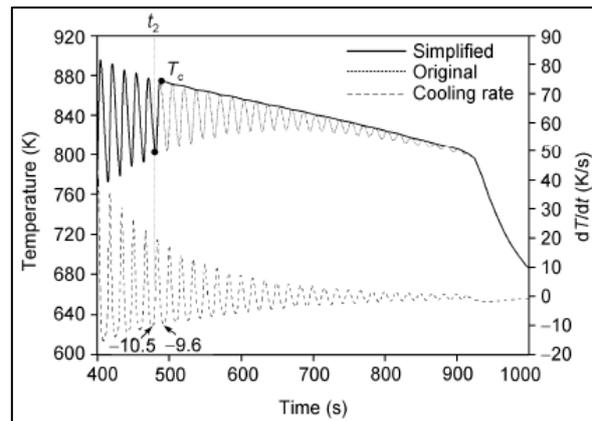
There is also a local minimum of  $T_c$  at the midpoint of each layer. This is because a short time interval of laser irradiations allows less thermal energy to be dissipated. As more layers are deposited, the energy accumulates and the whole temperature of the part increases.
