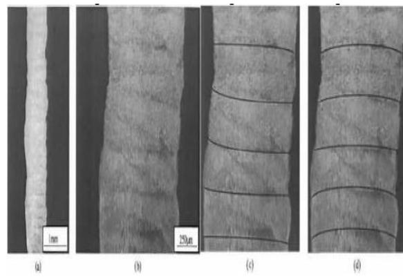
**Fig 21: Comparison of Melt Pool Boundaries Obtained by the Processing Result of the Edge Detector with Those Obtained by the Modelling, (a) Original Image Acquired by High Shutter Speed Camera, (b) Processing Result of Edge Detector, (c) Numerical Modelling Result, (d) Analytical Modelling Result [11]**
