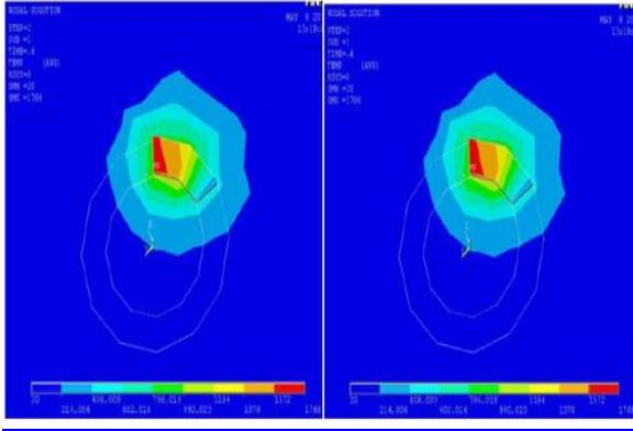
As can be seen from Figure 18 (a) (keeping power same) the molten pool temperature decreases with the radius, namely, the molten pool temperature increases with the curvature. It is also observed that the molten pool temperature tends to be gentle when the radius is more than 4 mm.
