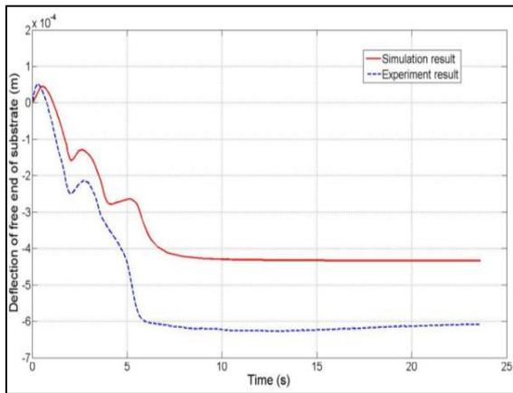
The process of DMD involves very high thermal gradients and heating and cooling rates, resulting in residual stresses and distortion, Heng Liu et al [13] presented a thermo-mechanical finite element model to predict residual stress and deformations. The thermal distribution, thermal stress field, geometry deformation and effect of deposition parameters on residual stress and deflections are explained.
