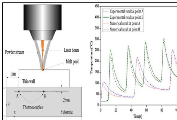
The temperature reached a peak every time the laser beam passed over the measuring point, and then decreased to a resident temperature. Thermal cycle period at point A was the double of that at point B. However, thermal history at the two points had the same changing trend.
