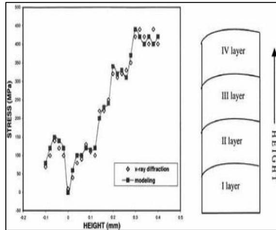
A three-step analytical and numerical approach was carried out by Peyre et al<sup>[12]</sup> to predict the shapes of manufactured structures and thermal loadings induced by the DMD process.
