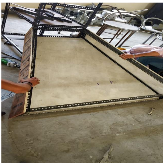
Figure 2: Wooden Planks Being Bolted with Collector Frame
