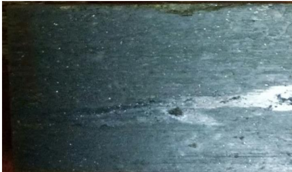
Figure 3: Brake Shoe Surface After Test
