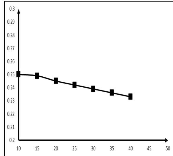
Figure 4 shows that exergetic efficiency of the system decreases with increasing ambient temperature. As the net workout from the micro-gas turbine decreases and the amount of heat carried by the exhaust gases increases with increasing ambient temperature therefore the output exergy of the system decreases however the heat of exhaust gases is being used by the VAR system and the output exergy is being recovered upto some extent.
