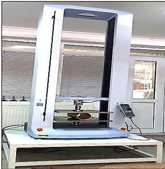
Fig 5: Dynamometer for Testing the Flexibility of the Ring Pipe Method
