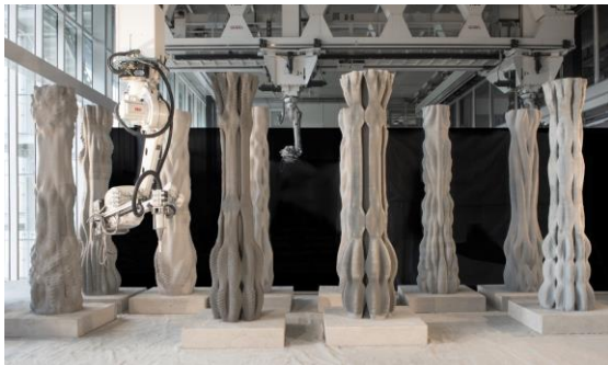
Figure 13: Concrete Pillars Made using Additive Manufacturing
