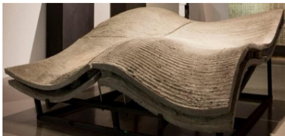
Figure 3: Curved Concrete Plate Made Using Additive Manufacturing
