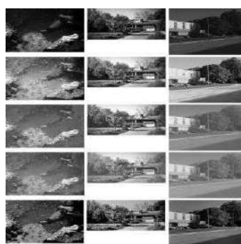
Figure 1: A comparison of the MSRCR with point operations. Top row: original; second row: histogram equalization; third row: gain/offset; fourth row: gamma non-linearity; bottom row: MSRCR
