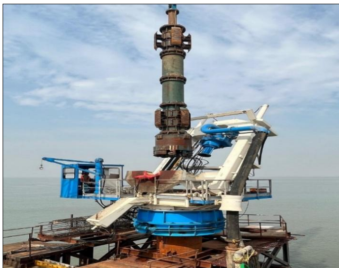
Figure 5: Drilling Setup and BHA Installation in RCD
